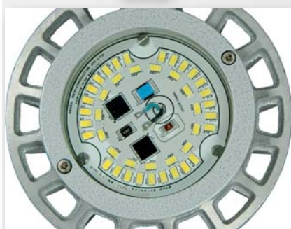
LED resin-bonded electronic board
